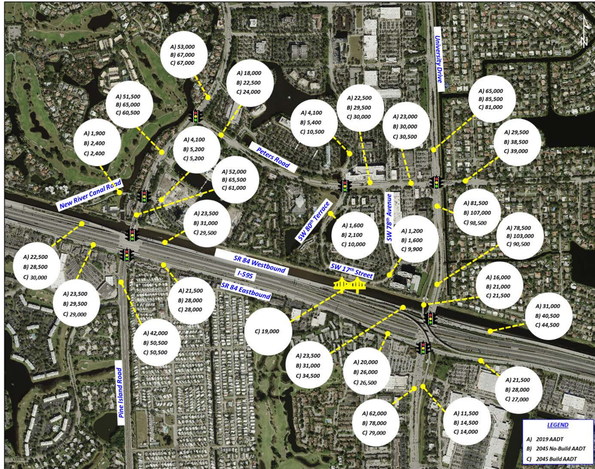
Figure 6: 2019 AADT, 2045 No Build AADT, and 2045 Build AADT
